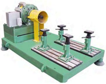
Engine Test Stands, Mounting Bed with T- slots having X, Y & Z adjustment for Length, Width & Height adjustments with mechanical / hydraulic jacks or scissor type lift platform with raise / lower lever & position lock, is supplied for Engine mounting with Cardan / Propeller shaft & adaptors between Engine and the loading device (Dynamometer) and necessary transducers. The test bench, being rigidly supported on four antivibration mounts.
