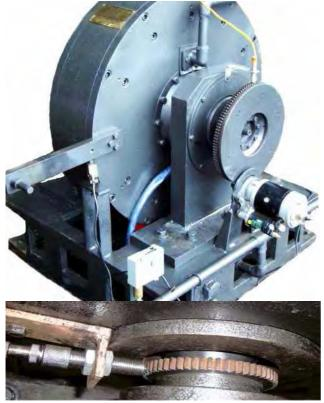
Eddy Current Dynamometer is Bi-directional, Dry-gap Type. Being Dry operation, the only resistance to movement of the rotor is bearing friction and the minimal windage effect. With zero excitation, an almost no-load condition is achieved over the entire speed range
